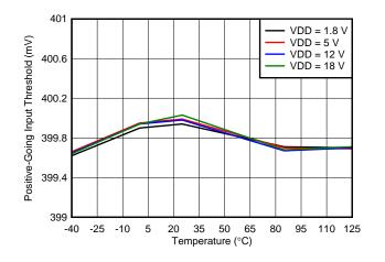
Figure 18. Rising Input Threshold Voltage (V<sub>IT+</sub>) vs Temperature
