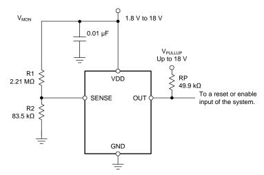
Figure 17. Wide VIN Voltage Monitor
