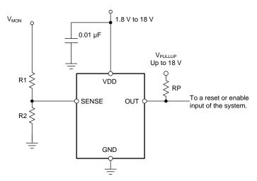
Figure 14. Interfacing to a Voltage Other Than V<sub>DD</sub>
