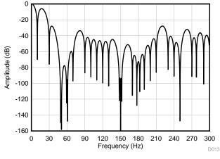
Figure 71. FIR Frequency Response (10 SPS)
