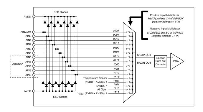
Figure 48. Analog Input Block Diagram
