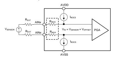
Figure 96. Burn-Out Current Source Offset Voltage Error
