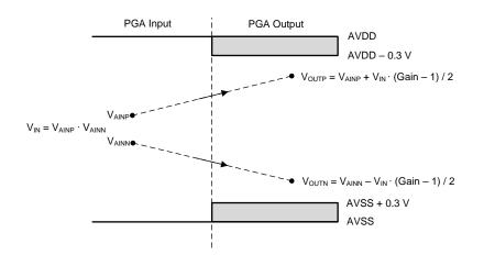
Figure 50. PGA Input/Output Range
