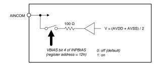
Figure 56. Level-Shift Voltage Diagram
