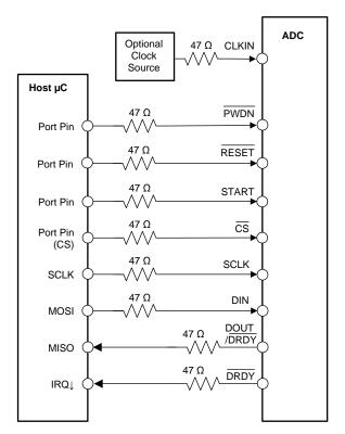
Figure 98. Serial Interface and Digital I/O Connections
