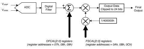
Figure 74. Calibration Block Diagram
