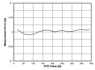
Figure 100. 3-Wire RTD Example Measurement Results
