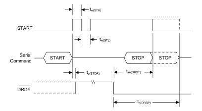
Figure 4. Conversion Control Timing Requirements
