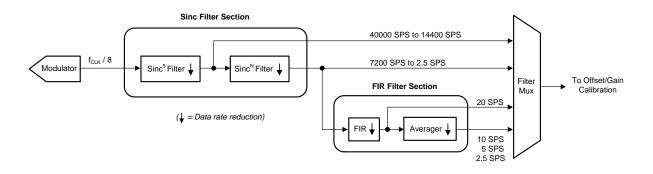
Figure 60. Digital Filter Block Diagram
