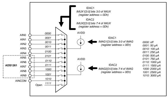
Figure 58. Current Source Connection
