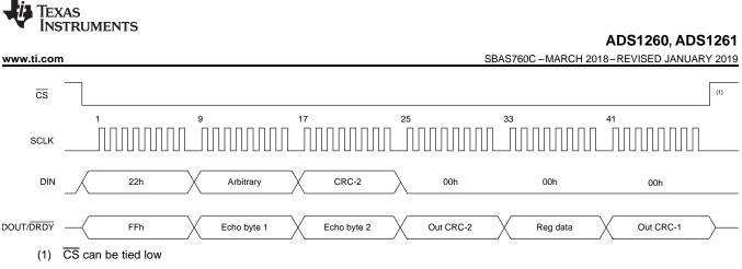
Figure 78. Register Read Operation (address = 02h, CRC Mode Enabled)
