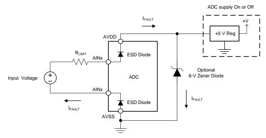
Figure 102. Analog Power-Supply Clamp
