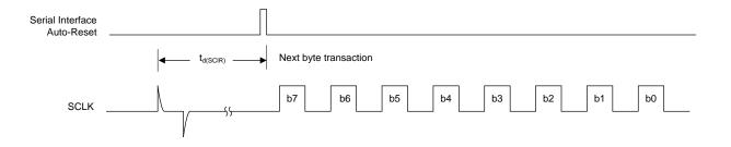
Figure 3. Serial Interface Auto-Reset Characteristics
