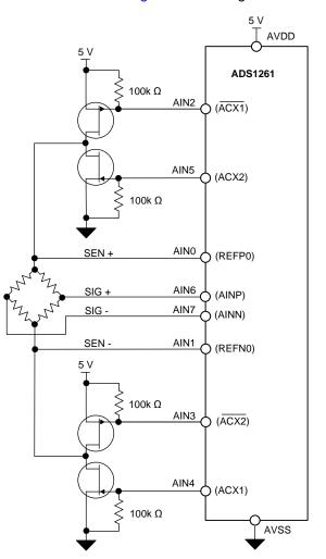
Figure 97. 4-Wire Drive, AC-Excitation Example
