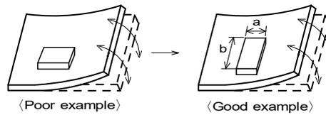
(2) Components location on PCB separation
