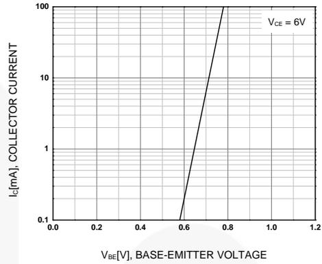
Figure 2. Transfer Characteristic
