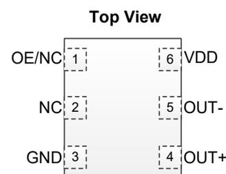
**Figure 3. Pin Assignments**
