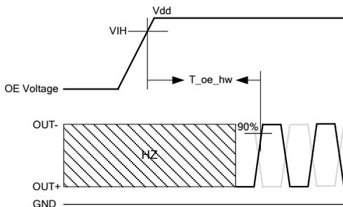
**Figure 8. Hardware OE Enable Timing**
