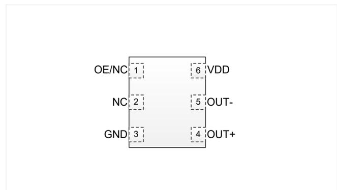
Figure 2. Pin Assignments (Top view)
