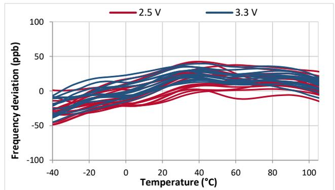
Figure 23. Frequency vs Temperature ( $\pm 0.1$  ppm), 105°C
