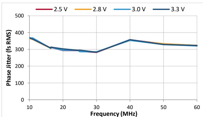
Figure 42. RMS Phase Jitter, DCTCXO, TCXO (Clip Sine)
