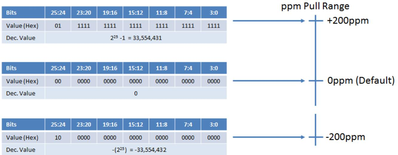
**Figure 52. Pull Range and Frequency Control Word**
