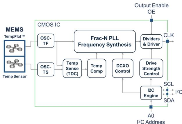
Figure 48. Block Diagram
