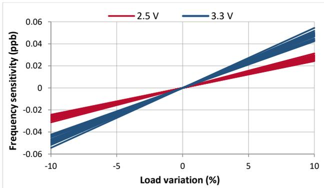
Figure 28. Load sensitivity ( $\pm 0.1$  ppm)
