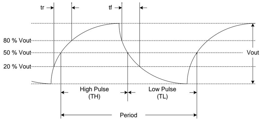
**Figure 16. Clipped Sinewave Waveform Diagram<sup>[13]</sup>**
