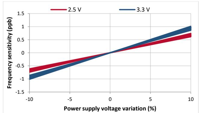
Figure 29. VDD sensitivity ( $\pm 0.1$  ppm)
