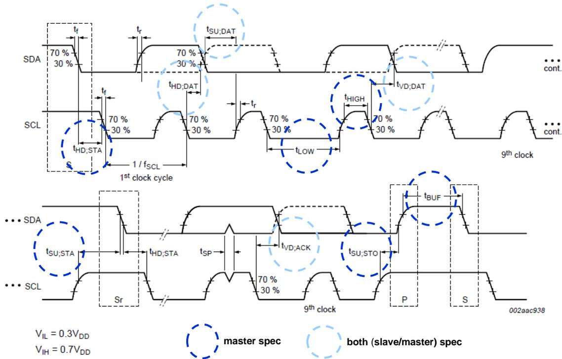
Figure 59. I<sup>2</sup>C Timing Diagram
