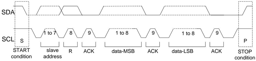
Figure 57. Parallel data byte format, read operation
