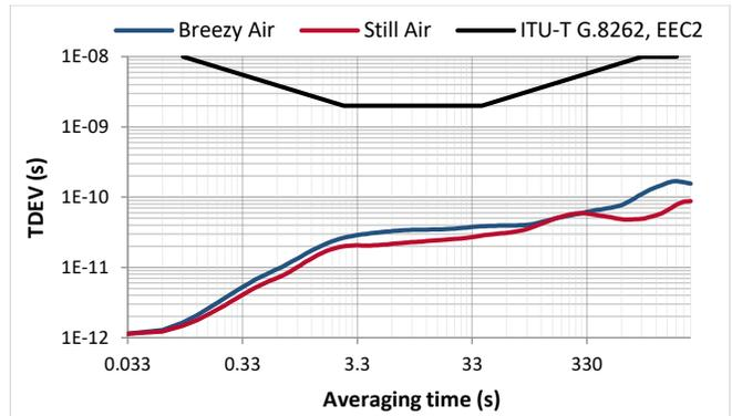
Figure 21. TDEV (0.1 Hz loop bandwidth,  $\pm 0.1$  ppm) [14]
