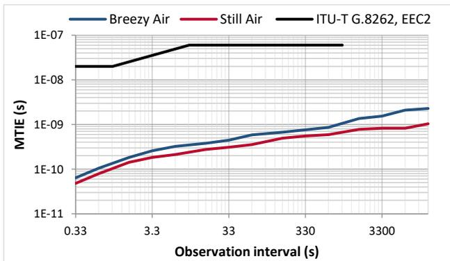
Figure 22. MTIE (0.1 Hz loop bandwidth,  $\pm 0.1$  ppm) [14]
