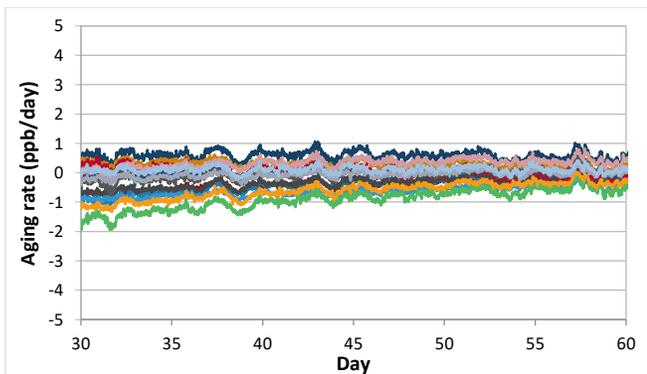
Figure 26. 1-day aging rate after 30 days, 0.1 ppm device
