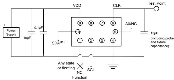
Figure 12. LVCMOS Test Circuit (I<sup>2</sup>C Control), DCTCXO mode for AC and DC Measurements
