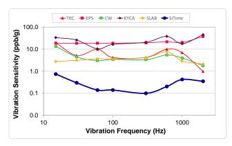
Figure 5. Vibration Robustness<sup>[5]</sup>
