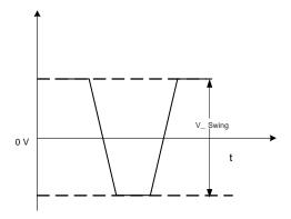
Figure 1(b). LVPECL Voltage Levels Across Differential Pair (i.e. OUT+ minus OUT-)
