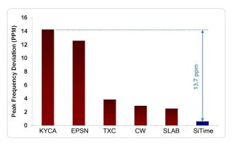
Figure 6. Shock Robustness<sup>[6]</sup>
