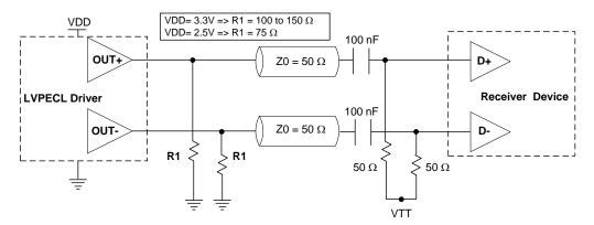
Figure 4. LVPECL AC Coupled Termination
