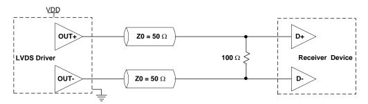
Figure 6. LVDS Single Termination (Load Terminated)
