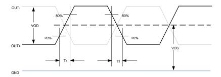
Figure 2. LVDS Voltage Levels per Differential Pin (i.e. OUT+, or OUT-)
