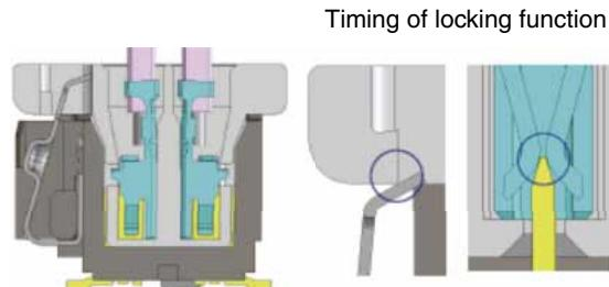
Simultaneous timing of locking function and contact mating provides a clearer tactile click.
