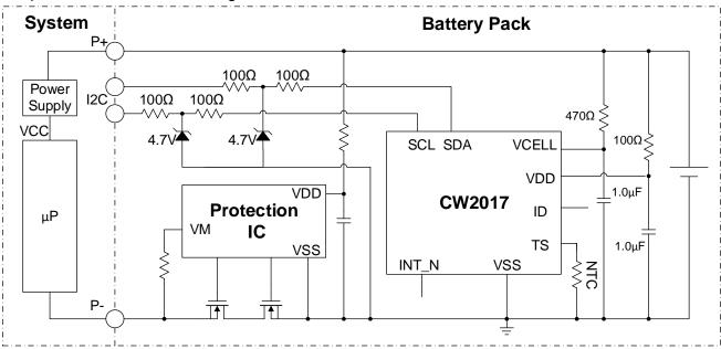
Figure 2. Typical Application Diagram (Pack Side)
