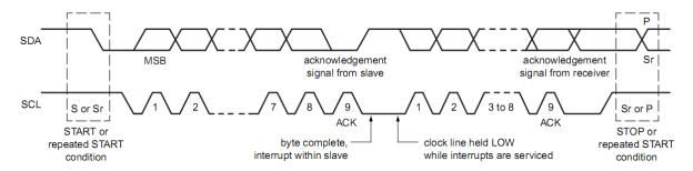
Figure 14. Data Transfer on the I2C Bus
