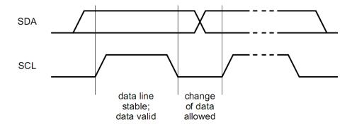
Figure 12. Bit Transfer on the I2C Bus
