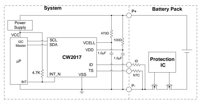
Figure 1. Typical Application Diagram (System Side)
