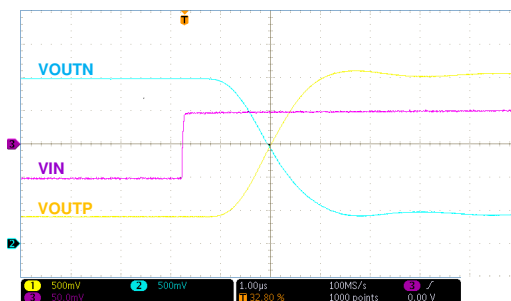
图 8-4. Step Response of the AMC1302
