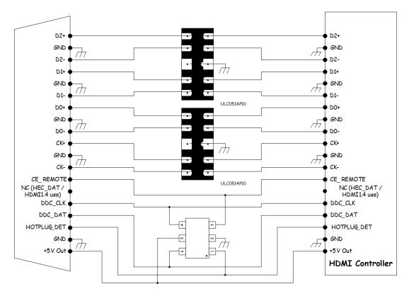
Figure 2. HDMI 2.0 Layout Diagram
