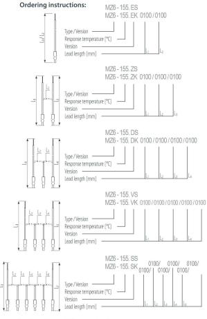
Version: ES: E-Single, S-Standard (520mm wire length) EK: E-single, K-custom, Z-dual, D-triple, V-quad, S-sixfold
