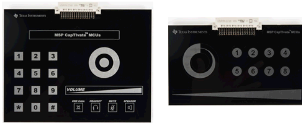
Figure 7-6. CAPTIVATE-PHONE and CAPTIVATE-BSWP Panels
