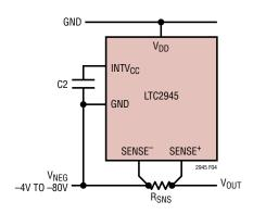
Figure 4. LTC2945 Derives Power from the Supply Being Monitored in Low-Side Current Sense Topology
