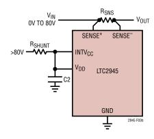
(b) Power Through Low-Side Shunt Regulator in High-Side Current Sense Topology
