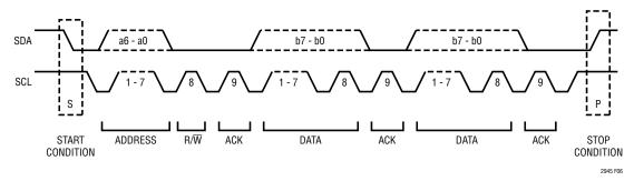
Figure 6. General Data Transfer Over I<sup>2</sup>C
