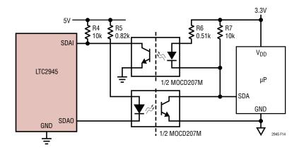
Figure 14. Opto-Isolation of a 10kHz I<sup>2</sup>C Interface Between LTC2945 and Microcontroller (SCL Omitted for Clarity)
