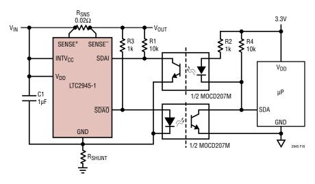
Figure 16. Low Speed 10kHz Opto-Isolators Powered from High-Side Shunt Regulator
