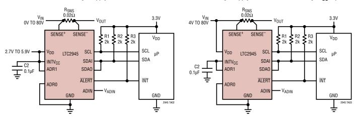
**Dual Supply Monitor with Common Opto-Coupler for Galvanic Isolation**
