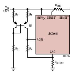
(a) Power Through High-Side Shunt Regulator
