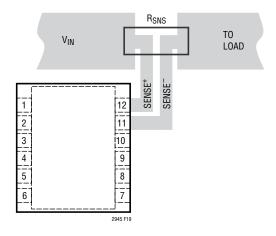
Figure 19. Recommended Layout for Kelvin Connection
