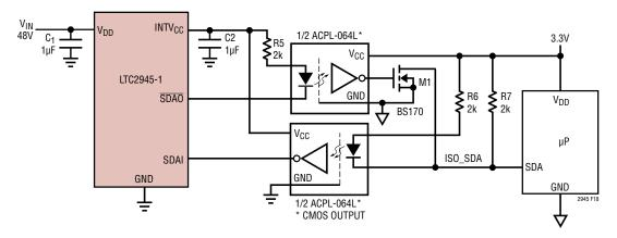
Figure 18. Opto-Isolation of I<sup>2</sup>C Interface with Low Power, High Speed Opto-Couplers (SCL Omitted for Clarity)
