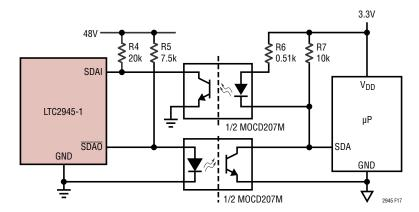
Figure 17. Opto-Isolation of a 1.5kHz I<sup>2</sup>C Interface Between LTC2945-1 and Microcontroller (SCL Omitted for Clarity)
