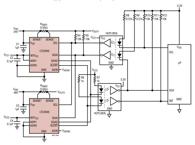
Power Monitoring in -48V System Using Low Side Sensing (1.5kHz I<sup>2</sup>C Interface)
