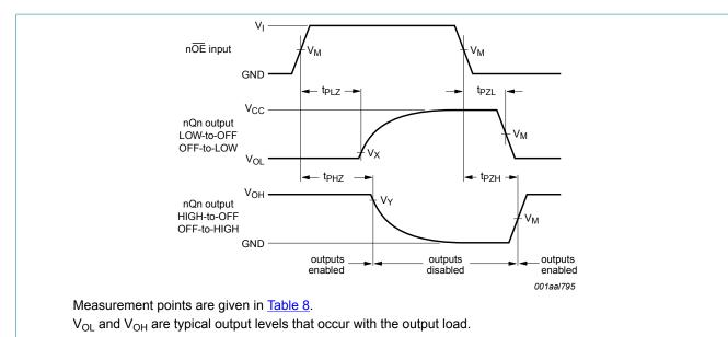
Fig. 8. 3-state enable and disable times
