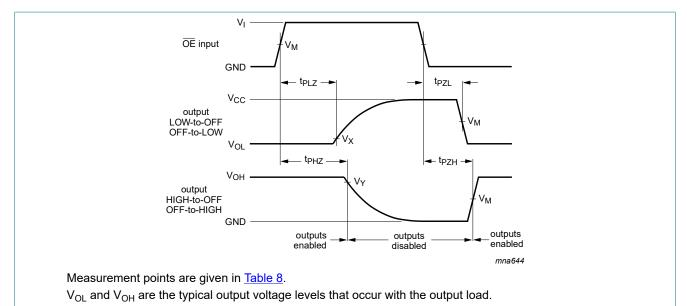
Fig. 8. Enable and disable times
