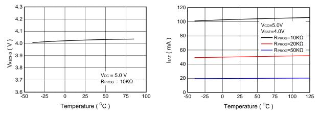
**Recharge Voltage Threshold vs Ambient Temperature Charge Current vs Ambient Temperature**
