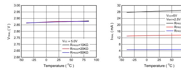
Trickle Charge Threshold vs Ambient Temperature Trickle Charge Current vs Ambient Temperature
