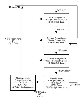
Figure 3. State Diagram of a Typical Charge Cycle
