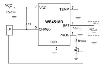
Figure 4. Manual Shutdown Mode Application Circuit
