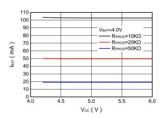
**Charge Current vs PROG Pin Voltage**
