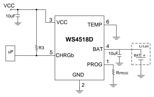
Typical applications W/T microprocessor detect
