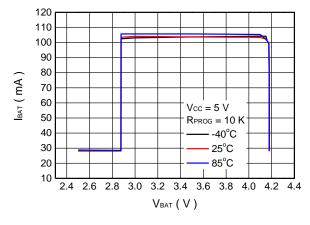
Float Voltage vs Ambient Temperature
