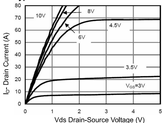
Figure 1 Output Characteristics
