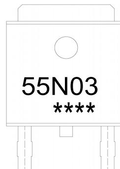
**Marking and pin assignment**
