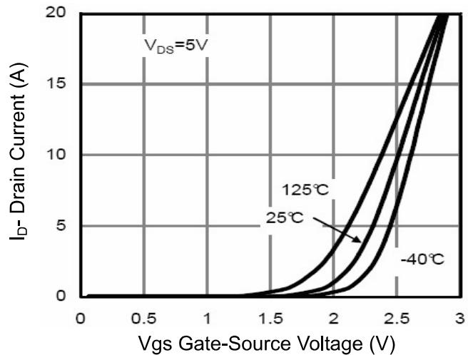
Figure 2 Transfer Characteristics
