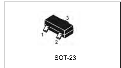
SOT-23 1: Ref; 2: Cathode; 3: Anode
