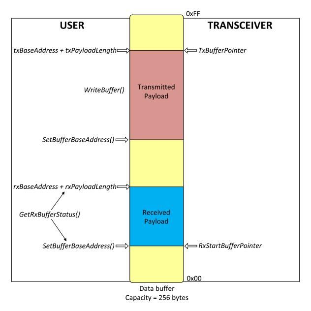
Figure 7-1: Data Buffer Diagram
