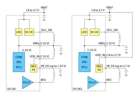
Figure 4-3: PA Supply Scheme in DC-DC Mode
