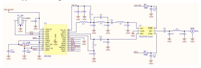
Figure 14-2: Application Schematic of the SX1262 with RF Switch
