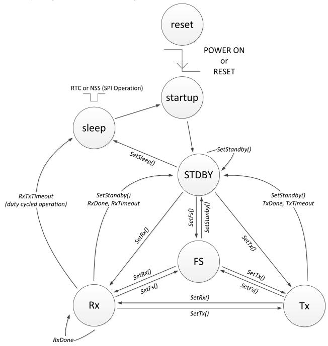
**Figure 9-1: Transceiver Circuit Modes**
