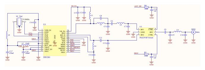
Figure 14-1: Application Schematic of the SX1261 with RF Switch
