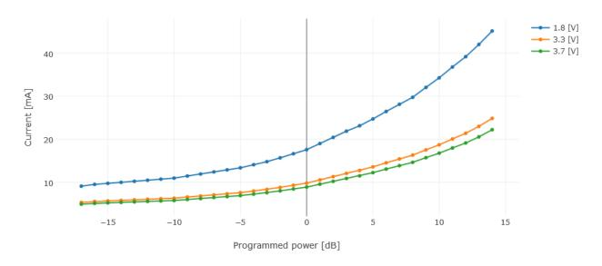
Figure 4-5: Current versus Output Power with DC-DC Regulation on the SX1261
