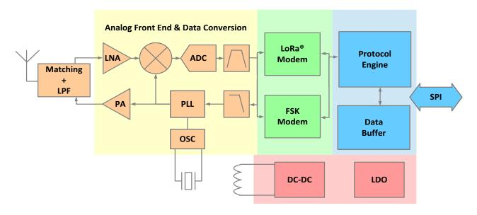
Figure 4-1: SX1261/2 Block Diagram
