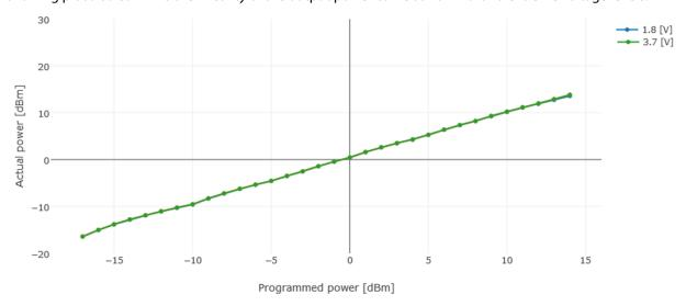
Figure 4-7: Power Linearity on the SX1261 with either LDO or DC-DC Regulation
