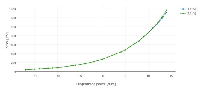
Figure 4-4: VR\_PA versus Output Power on the SX1261
