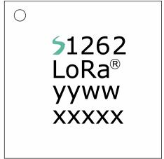
Marking for the 4 x 4 mm MLPQ 24 Lead package:
