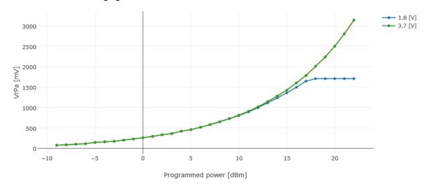
Figure 4-8: VR\_PA versus Output Power on the SX1262
