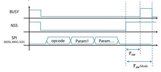
Figure 8-4: Switching Time Definition in Active Mode
