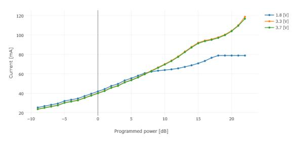
Figure 4-10: Current versus Programmed Output Power on the SX1262
