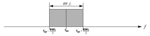
Figure 6-1: LoRa® Signal Bandwidth
