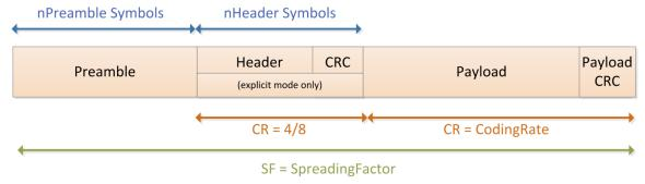
Figure 6-2: LoRa® Packet Format
