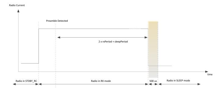
Figure 13-3: RX Duty Cycle when Receiving
