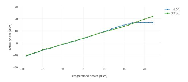
Figure 4-9: Power Linearity on the SX1262
