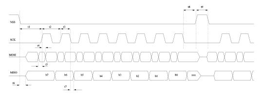
Figure 8-1: SPI Timing Diagram
