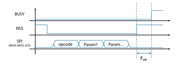
Figure 8-3: Switching Time Definition
