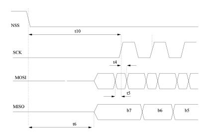
**Figure 8-2: SPI Timing Transition**
