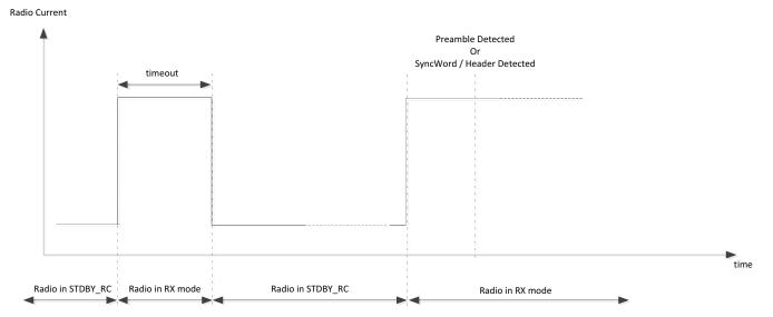
Figure 13-1: Stopping Timer on Preamble or Header Detection
