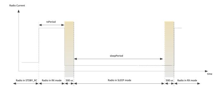
Figure 13-2: RX Duty Cycle Energy Profile
