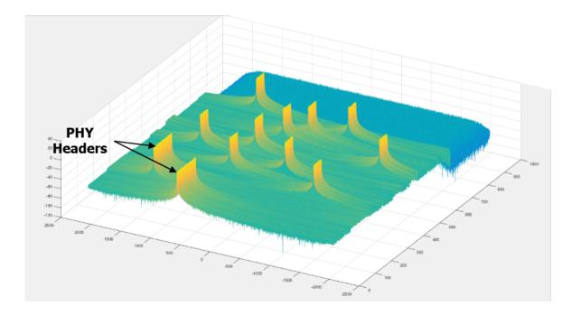
Figure 6-6: LR-FHSS Example Spectral Plot
