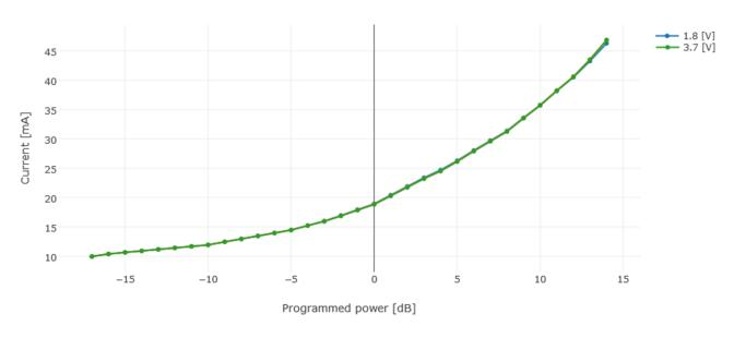
Figure 4-6: Current versus Output Power with LDO Regulation on the SX1261
