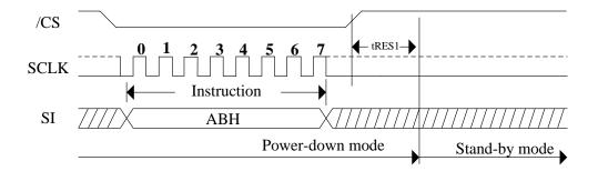
Figure 15b. Release Power-Down/Read Device ID Sequence Diagram
