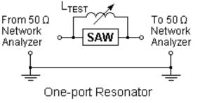
The test circuit inductor,  $L_{TEST}$ , is tuned to resonabte with the static capacitance,  $C_0$  at  $f_C$ .
