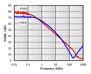
Figure 20. CMRR and PSRR vs. Frequency
