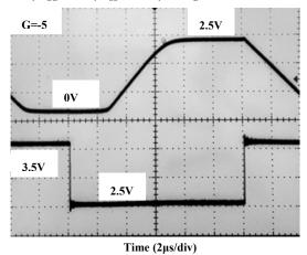
Figure 13. Positive Overload Recovery Time
