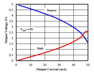
Figure 9. Output Voltage vs. Output Current
