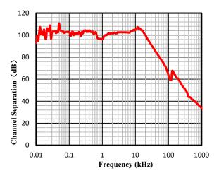
Figure 21. Channel Separation vs. Frequency
