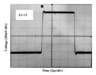
Figure 17. Small-Signal Step Response
