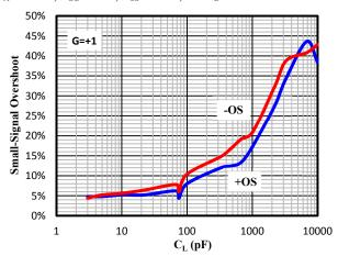
Figure 7. Small-Signal Overshoot vs. Load Capacitance
