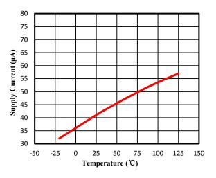
Figure 2. Supply Current vs. Temperature
