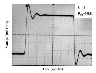
Figure 18. Small-Signal Step Response
