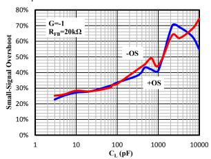
Figure 8. Small-Signal Overshoot vs. Load Capacitance
