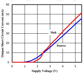
Figure 3. Output Short Circuit Current vs. Supply Voltage
