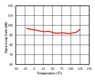
Figure 4. Open-Loop Gain vs. Temperature
