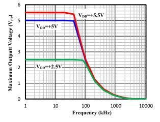
Figure 12. Maximum Output Voltage vs. Frequency
