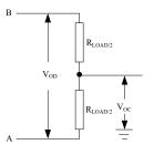
Figure 2. Driver DC Test Load
