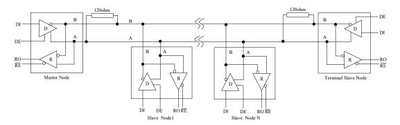
Figure 1. Typical Half-Duplex RS-485 Network
