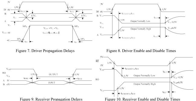
Figure 9. Receiver Propagation Delays
