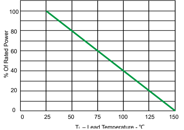
Fig 2. Power Derating Curve
