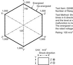
Test Item: G5NB-1A, 24VDC Number of Relays: 5 pcs Test Method: Shock is applied 3 times in 6 directions along 3 axes and the level at which shock caused malfunction is measured. The energized voltage is 100% of the rated voltage. Rating: 100 m/s<sup>2</sup>
