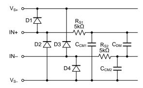
Figure 1. Input EMI Filter and Clamp Circuit
