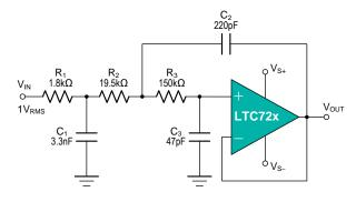
Figure 6. Configured as a Three-Pole, 20-kHz, Sallen-Key Filter
