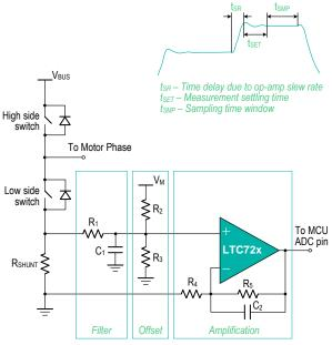
Figure 7. Current Shunt Monitor Circuit
