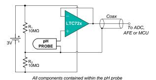
Figure 10. Buffered pH Probe
