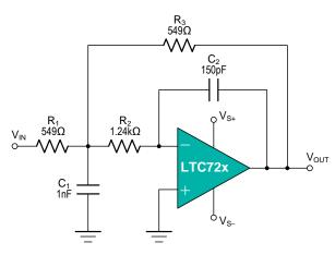
Figure 5. Second-Order, Butterworth, 500-kHz Low-Pass Filter
