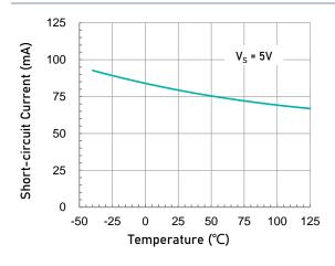
Short-circuit Current as a function of Temperature.
