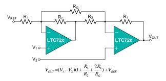
Figure 9. Instrumentation Amplifier
