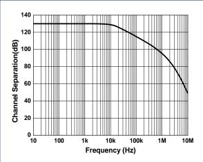
Channel Separation as a function of Frequency.
