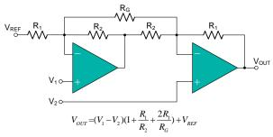
Figure 6. Instrumentation Amplifier
