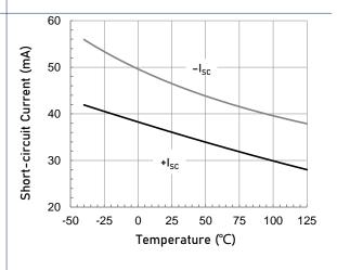
Short-circuit Current as a function of Temperature.
