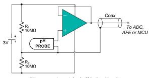
All components contained within the pH probe
