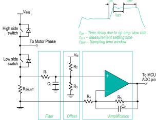
Figure 8. Current Shunt Monitor Circuit
