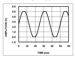
Figure 2. No Phase Inversion with Inputs Greater Than the Power-Supply Voltage
