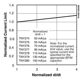
Figure 23. Current Limit vs. di/dt.
