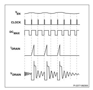
Figure 8. Operation at Medium Loading.
