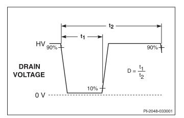
Figure 17. Duty Cycle Measurement.
