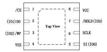
Figure 3.2. Pin Configuration DFN 4\*3mm
