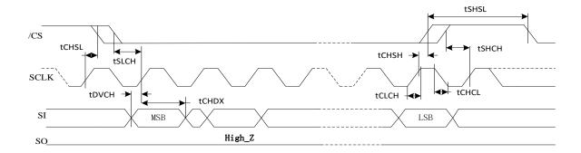
Figure 47. Output Timing
