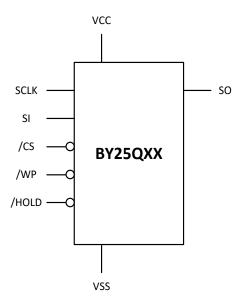
Figure 2. Pin Configuration SOP8
