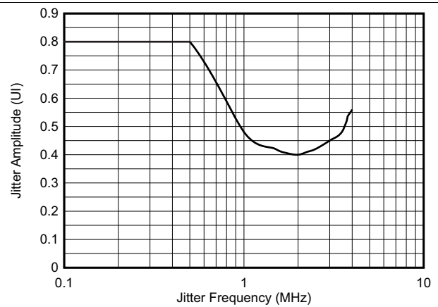
Figure 12. Typical System Input Jitter Tolerance Curve - DS90UB913A Linked to DS90UB914A
