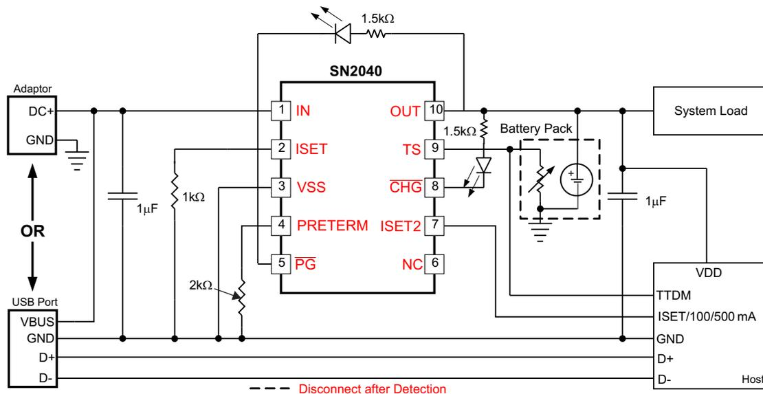
**Figure 14. Typical Application Circuit**
