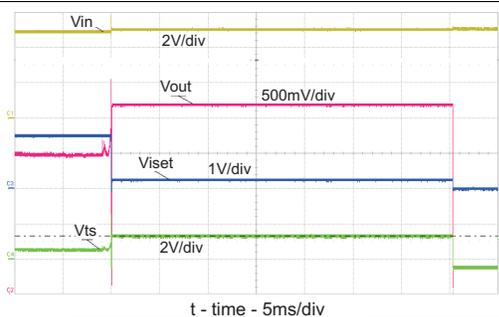
Figure 23. Battery Removal – GND Removed 1st, 42 Ω Load
