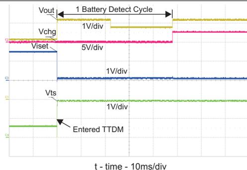
Figure 24. Battery Removal with OUT and TS Disconnect 1st, With 100 Ω Load
