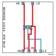
Max  $R_{\theta JA} = 140 ^{\circ} C/W$  when mounted on minimum pad area of 2 oz. (0.071 mm thick) Cu.
