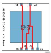
Max  $R_{\theta JA} = 76^{\circ} C/W$  when mounted on 1 inch² (6.45 cm²) of 2 oz. (0.071 mm thick) Cu.
