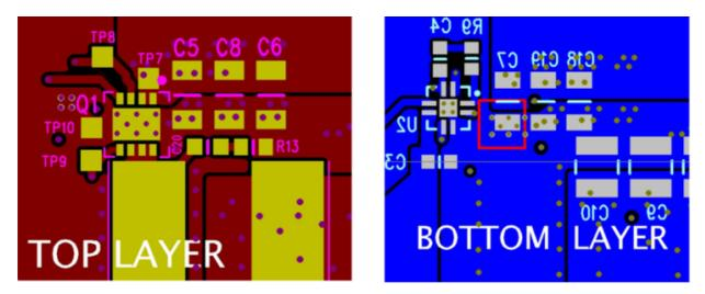
Figure 34. Recommended PCB Layout (Top Down)
