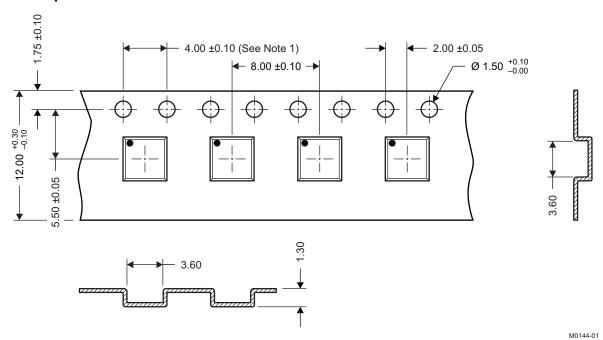
NOTES: 1. 10-sprocket hole-pitch cumulative tolerance ±0.2
