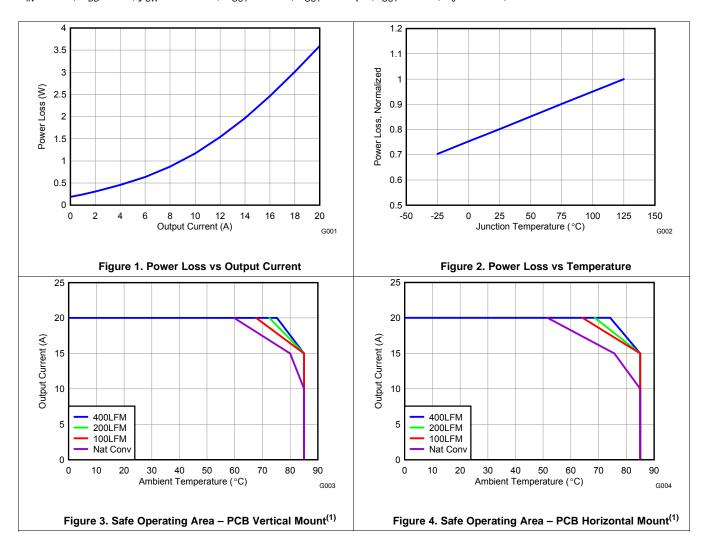
(1) The Typical Power Block System Characteristic curves are based on measurements made on a PCB design with dimensions of 4.0" (W) × 3.5" (L) × 0.062" (H) and 6 copper layers of 1 oz. copper thickness. See Application Section for detailed explanation.
