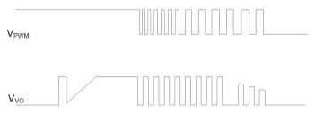
Figure 1 PWM Input Waveform
