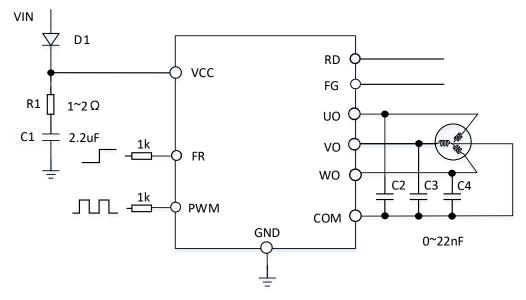
Note1: D1 is to prevent the damage from the power reverse connection.
