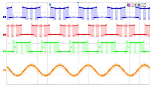
$CH1: V_{UO}, 5V/div, DC\;; \quad CH2: V_{VO}, 5V/div, DC; \quad CH3: V_{WO}, 5V/div, DC; \quad CH4: I_{UO}, 200mA/div, DC$
