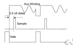
The auxiliary winding voltage is a well-defined replica of the output voltage. The OVP works by sampling the plateau voltage at CS pin during the flyback phase. OB2365D can sample this flat voltage level after a delay time to perform over temperature protection. This delay time is used to
