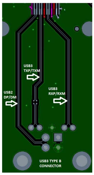
图 58. Example Routing of Upstream Port
