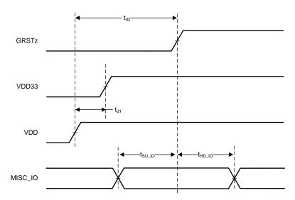
图 1. Power-Up Timing Requirements
