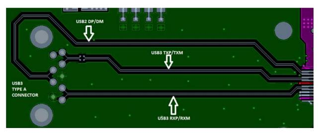
图 59. Example Routing of Downstream Port
