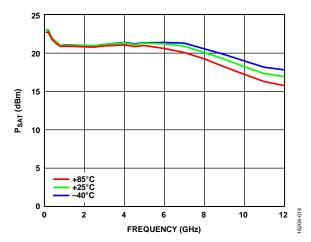
Figure 14. Saturation Power (P<sub>SAT</sub>) vs. Frequency at Various Temperatures
