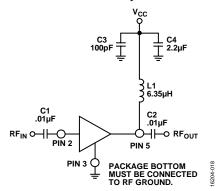
Figure 18. Evaluation Board Schematic
