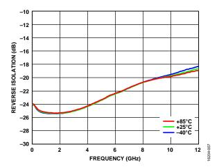
Figure 7. Reverse Isolation vs. Frequency at Various Temperatures
