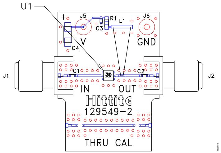
Figure 19. Evaluation Board, Top View
