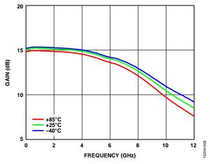
Figure 8. Gain vs. Frequency at Various Temperatures
