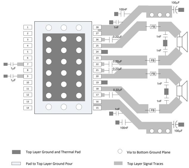
Figure 27. BTL Layout Example
