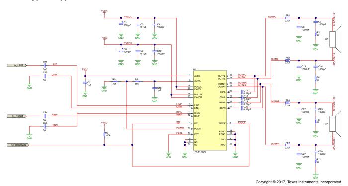
Figure 18. Stereo Class-D Amplifier with BTL Output and Single-Ended Inputs with Spread Spectrum Modulation
