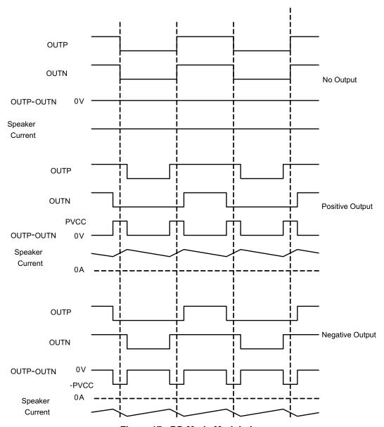
Figure 17. BD Mode Modulation
