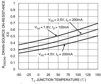
Figure 7. On-Resistance Variation with Temperature
