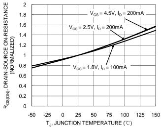
Figure 6. On-Resistance Variation with Temperature
