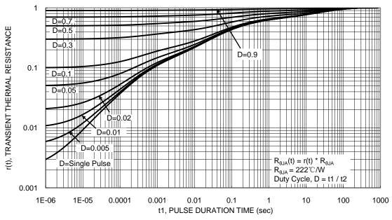
Figure 13. Transient Thermal Resistance
