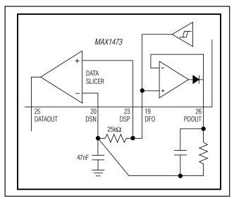
Figure 4. Using PDOUT for Faster Startup
