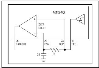
Figure 2. Generating Data Slicer Threshold
