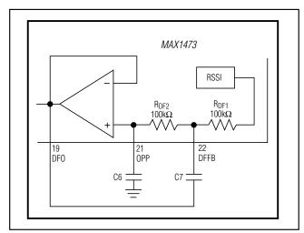
Figure 1. Sallen-Key Lowpass Data Filter
