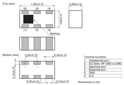
Note Pin 2 of the filter provides a DC feed connection to the balanced ports. In the event that this function is used, Pin 2 should be connected to ground using a de-coupling capacitor.
