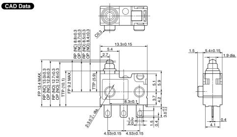
**3. Angle terminal type (3 mm standard type only)** Right type
