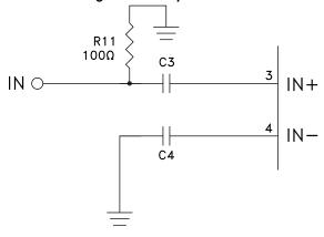
Choose the input decoupling capacitor (C3, C4) values by first determining the lowest spectral component the power detector is required to sense, *f*L.
