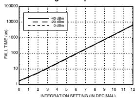
For increased load drive capability, consider a buffer amplifier on the RMS output. Using an integrating amplifier on the RMS output allows for an alternative treatment for faster settling times. An external amplifier optimized for transient settling can also provide additional RMS filtering, when operating HMC909LP4E with a lower SCI value.
