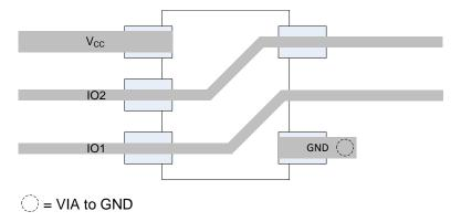
Figure 6. Routing With DRL Package
