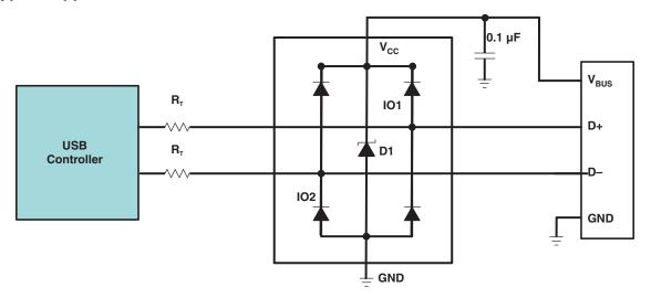
Figure 5. Typical USB Application Diagram
