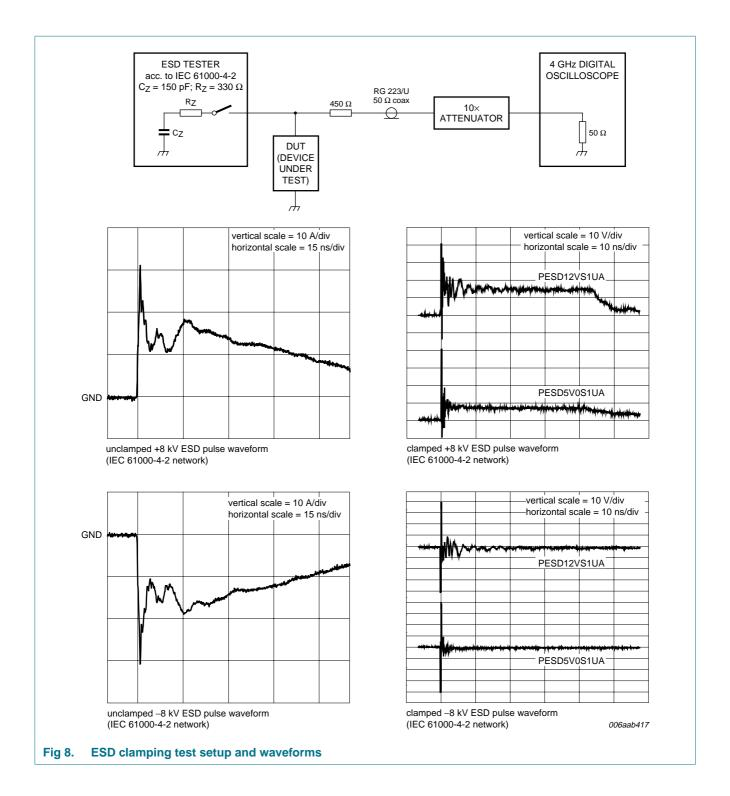
Unidirectional ESD protection for transient voltage suppression
