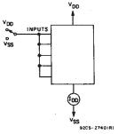
Fig. 13 — Quiescent device current test circuit.
