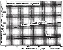
Fig. 10 — Typical propagation delay time as a function of load capacitance  $(\phi \text{ to } Q_1)$ .
