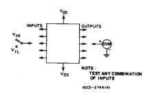
Fig. 14 - Input voltage test circuits.
