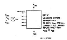
Fig. 15 - Input current test circuit.
