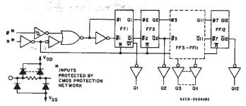
Fig. 3 - Logic diagram for CD4040B.
