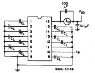
Fig. 12 – Dynamic power dissipation test circuit for CD4020B.
