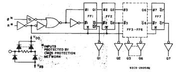
Fig. 2 - Logic diagram for CD4024B.
