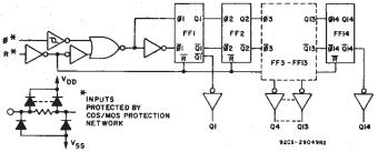
Fig. 1 - Logic diagram for CD40208.
