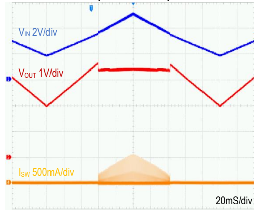
100% Duty Cycle Entry and Leave Operation V_{IN}=2\text{V to }5\text{V}, V_{OUT}=3.3\text{V}, I_{OUT}=10\text{mA}
