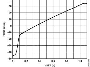
Figure 42. POUT vs. VSET at 0.9 GHz for Single Mode Handset
