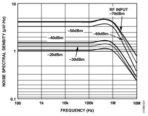
Figure 21. V<sub>DN</sub> Noise Spectral Density
