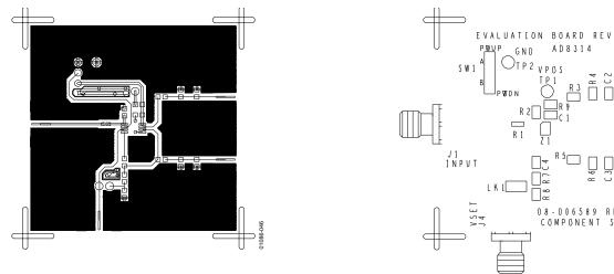
Figure 46. Layout of Component Side (MSOP)
