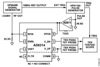
Figure 24. Test Setup for Power-On and Power-Off Response
