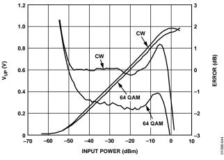
Figure 44. Shift in Transfer Function due to 64 QAM
