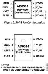
Figure 3. CP-8-23 Pin Configuration
