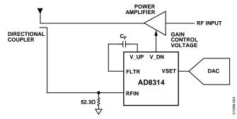
Figure 34. Typical Controller Mode Application
