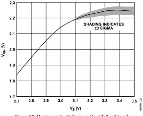
Figure 25. Maximum  $V_{DN}$  Voltage vs. V<sub>s</sub> with 3 mA Load
