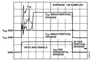
Figure 23. Power-On and Power-Off Response, Measurement Mode
