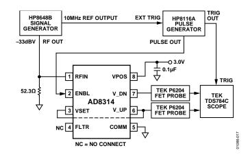
Figure 17. Test Setup for ENBL Response Time
