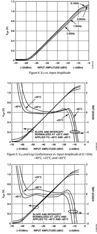
Figure 6. VuP and Log Conformance vs. Input Amplitude at 0.9 GHz; -40°C, +25°C, and +85°C
