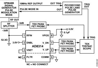
Figure 20. Text Setup for Pulse Response
