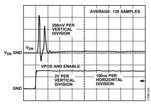
Figure 26. Power-On Response,  $V_{DN}$ , Controller Mode with VSET Held Low
