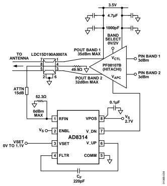
Figure 39. A Dual Mode Power Amplifier Control Circuit
