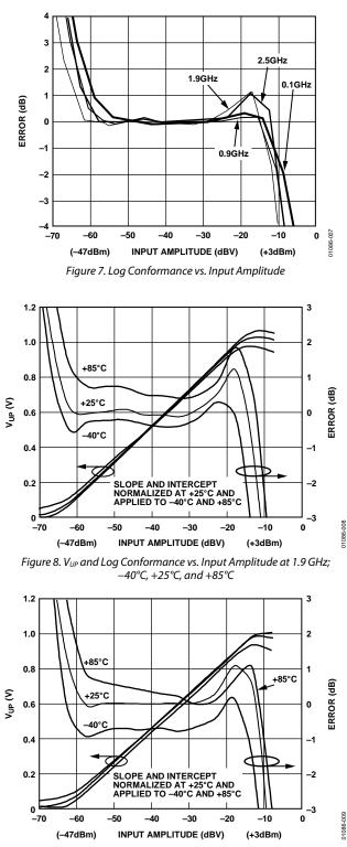
Figure 9. Vup and Log Conformance vs. Input Amplitude at 2.5 GHz; -40°C, +25°C, and +85°C
