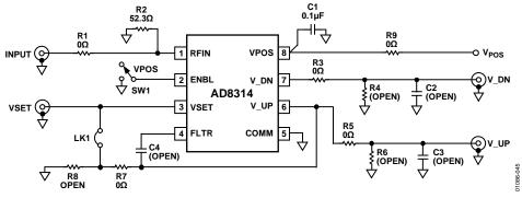
Figure 45. Evaluation Board Schematic
