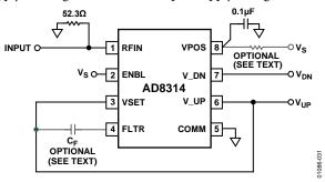
Figure 31. Basic Connections for Operation in Measurement Mode
