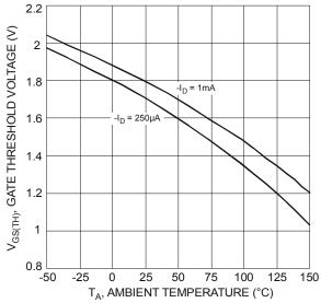
Figure 19 Gate Threshold Variation vs. Ambient Temperature
