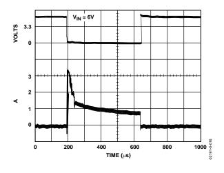
Figure 16. Short-Circuit Current
