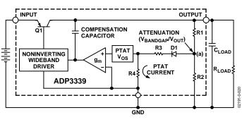
Figure 21. Functional Block Diagram
