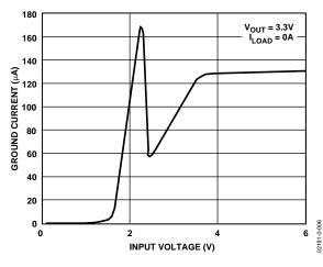
Figure 6. Ground Current vs. Supply Voltage
