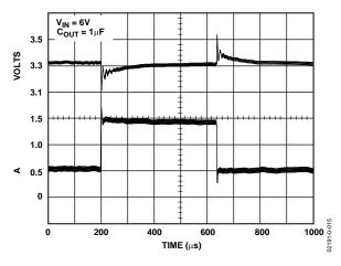
Figure 15. Load Transient Response
