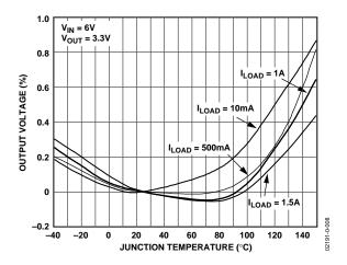
Figure 8. Output Voltage Variation Percentage vs. Junction Temperature
