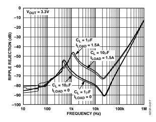
Figure 17. Power Supply Ripple Rejection
