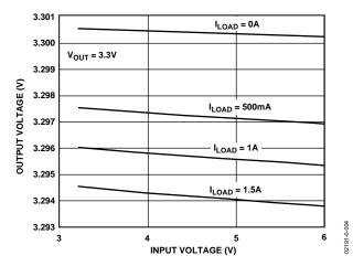
Figure 4. Output Voltage vs. Input Voltage
