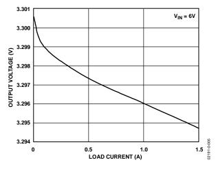
Figure 5. Output Voltage vs. Load Current
