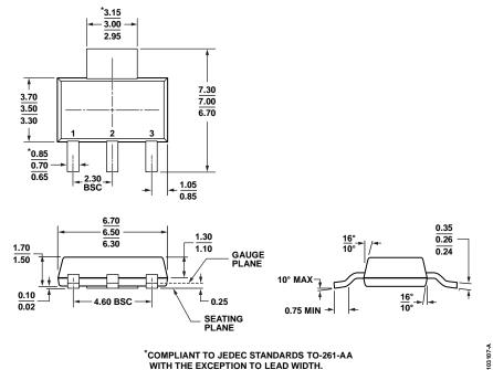
\*COMPLIANT TO JEDEC STANDARDS TO-261-AA WITH THE EXCEPTION TO LEAD WIDTH. Figure 23. 3-Lead Small Outline Transistor Package [SOT-223] (KC-3) Dimensions shown in millimeters
