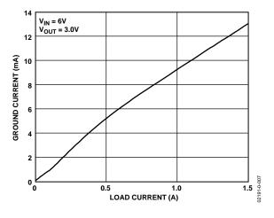
Figure 7. Ground Current vs. Load Current
