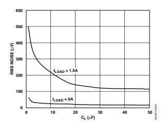
Figure 18. RMS Noise vs. CL (10 Hz to 100 kHz)
